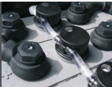
"A-version": automatic filling system on the basis of filler caps and floats. Advantage: all cells are simultaneously refilled in an instant and without spilling up to the right level: time-saving!
