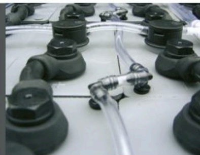
"Z-version": Acid circulation version, cells with acid circulation. Every element contains a little tube in which the charger pumps a little quantity of air which makes the electrolyte circulate from the beginning of the charge (cf diagram)
